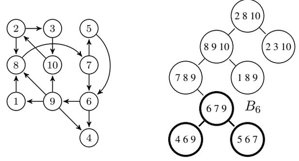
Figure 2: A graph  $G$  with treewidth 2 (left) and a corresponding tree-decomposition  $T = \text{Tree}(G)$  of 8 bags and width 2 (right). The distinguished bag  $B_6$  is the root bag of node 6. We have  $V_T(B_6) = \{6, 7, 9, 4, 5\}$  and  $\mathcal{V}_T(B_6) = \{6, 7, 9, 8, 10, 2\}$ . The subtree  $T(B_6)$  is shown in bold.
